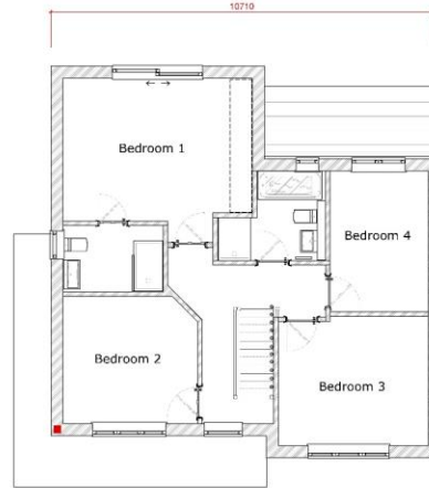
PROPOSED FIRST FLOOR PLAN. plot 5
